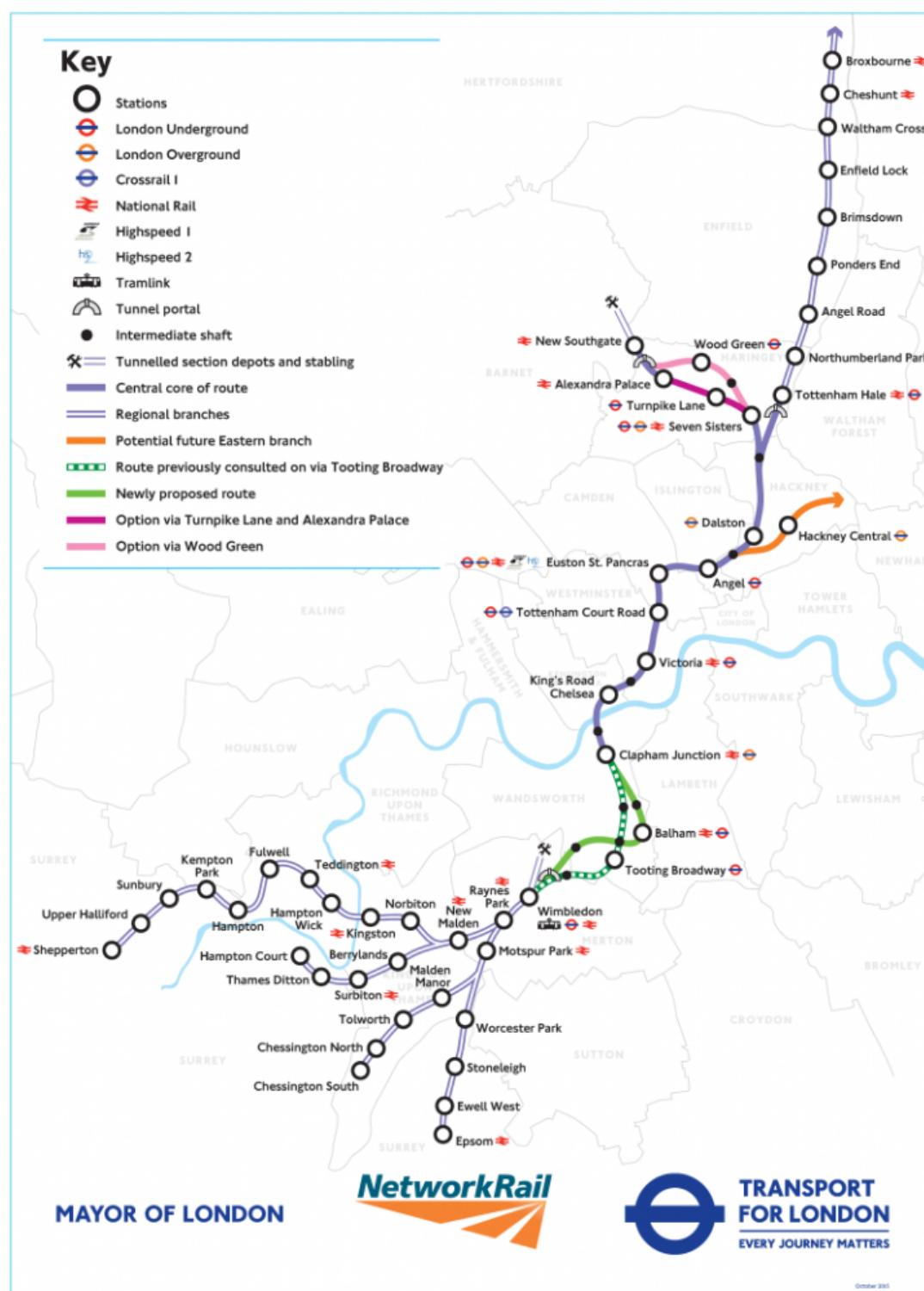
The proposal is for a new line in a tunnel from just north of Wimbledon via either Tooting or Balham to Clapham Junction then Kings Road, Chelsea, Victoria, Tottenham Court Road, Euston/St Pancras, then Angel and north from there to Tottenham Hale and New Southgate. The black dots on the map are intermediate shafts for building access.
